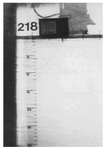
FIGURE 6. Formation of double-diffusive layers due to sidewall heating at t' = 46 min in doubly stratified experiment 218.
